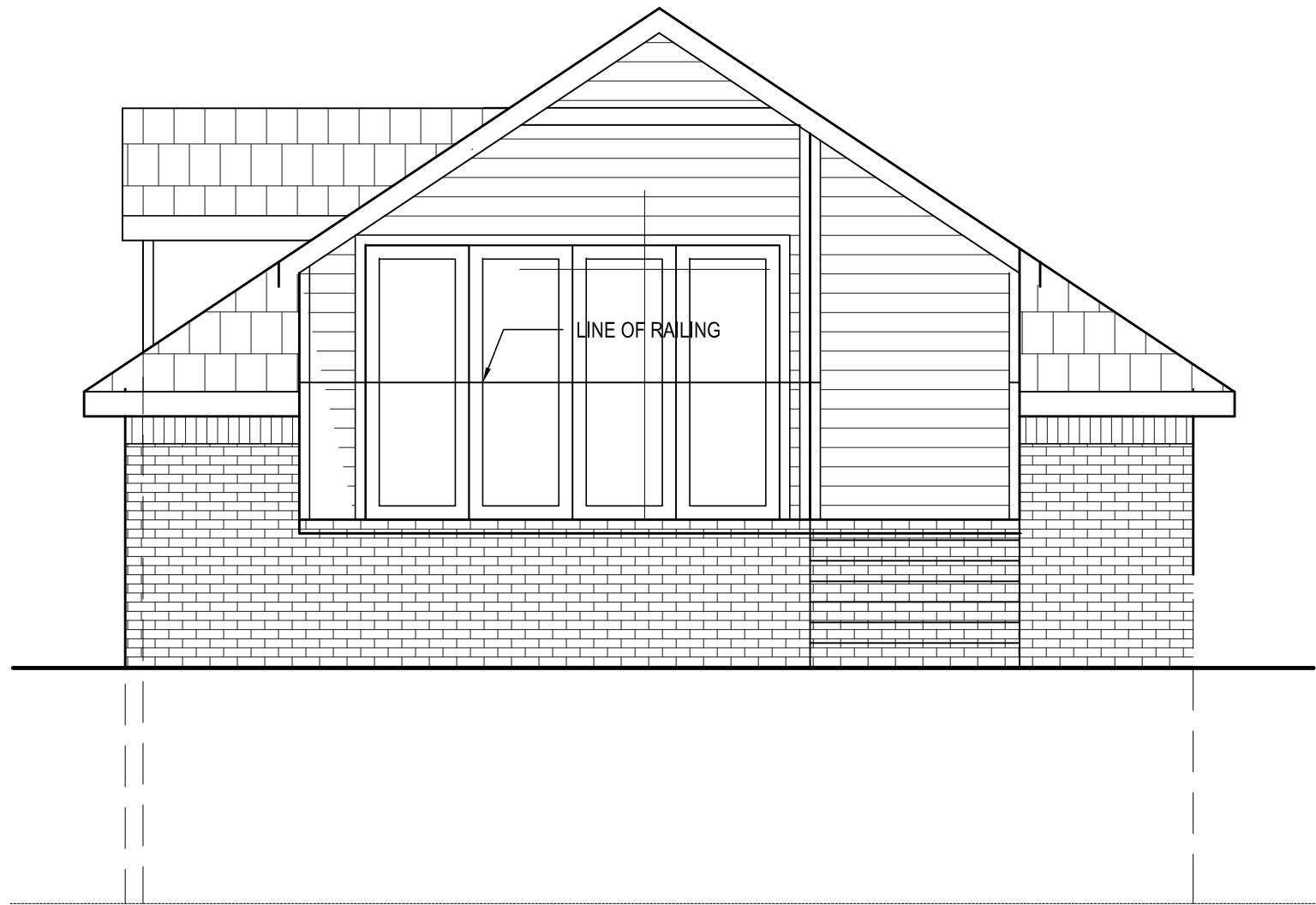
4 EAST ELEVATION ALTERNATE - GARAGE / POOL HOUSE 1/4" = 1'-0"
